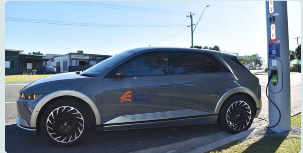
Essential Energy's pole-mounted EV charger trial in Kew used existing infrastructure to deliver accessible, future-ready charging.
